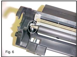
6. Assemble the PCR by pushing the PCR ends into the saddles (Fig. 6).
