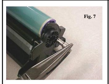
**10.** To remove the OPC axle and allow for replacement of the drum, twist and pull the exposed end until disengaged.
