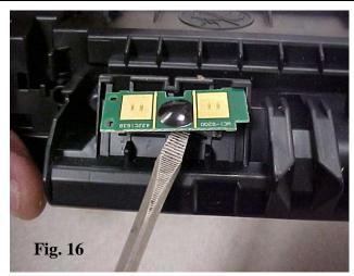
**NOTE:** After rebuilding the toner, it is necessary to install a replacement chip.
