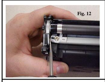
**NOTE:** The side cap has a small alignment post that is ultrasonically welded to the hopper body.
