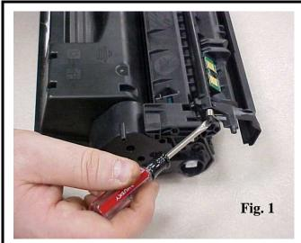
1. To separate the cartridge sections, first remove the OPC protective shutter by inserting a small flathead screwdriver under the end of the shutter arm and pry up.
