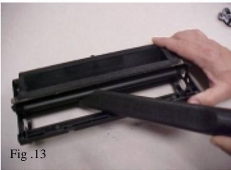
13. Clean the developer roller as well as the sponge roller with compressed air. It is not recommended to remove the Dr. Bar assembly because of the possibility of damaging the sealing foam (Fig. 13). After reinstalling all components in reverse order, fill hopper with toner then replace top cover.
