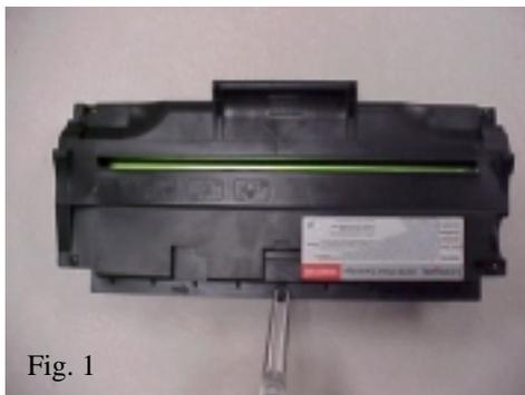
1. With end-clippers cut and remove the small plastic wall surrounding the center locking screw. Using the needle-nose pliers remove the screw and replace it with a #2 self-tapping screw before re-assembly (Fig 1).
