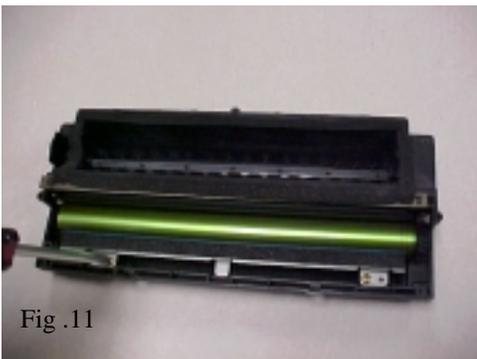
11. Remove the two screws that hold the foam PCR cleaner in place. **CAUTION:** there is a thin piece of urethane that acts as a wiperblade attached to the underside of the cleaning bar, do not damage this component when removing the cleaning bar.
