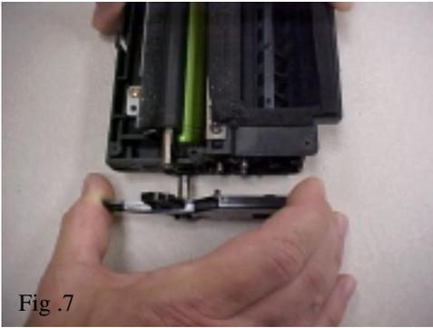
7. End plate removal. Pcr will remain in place until other end cap is removed (Fig 7).
